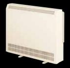
Off-peak storage heating takes advantage of cheap night time tariffs to provide an economical cost-effective heating system. Having stored heat on the cheap night off-peak tariff, the storage heater is designed to gradually release the stored heat throughout the day. If sized correctly, the storage heater will maintain room temperature at a comfortable level over a 24 hour period.
